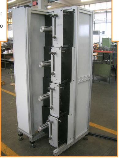
The traversing take up AV 4X220 CA 60 is a multiple take-up with independent spindle. It is equipped with a PLC which allows to program the steps of distribution of tapes with controlled tension. The possible settings are: continuous spiral, step by step, step fixed, regular or bi-conical flanges.
